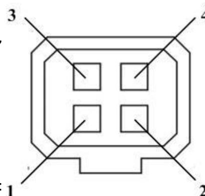
Auto iris interface with video driving uses three pins: Power, Video and GND; Auto iris interface with DC driving uses four pins: Damp+, Damp-, Drive+ and Drive-.
