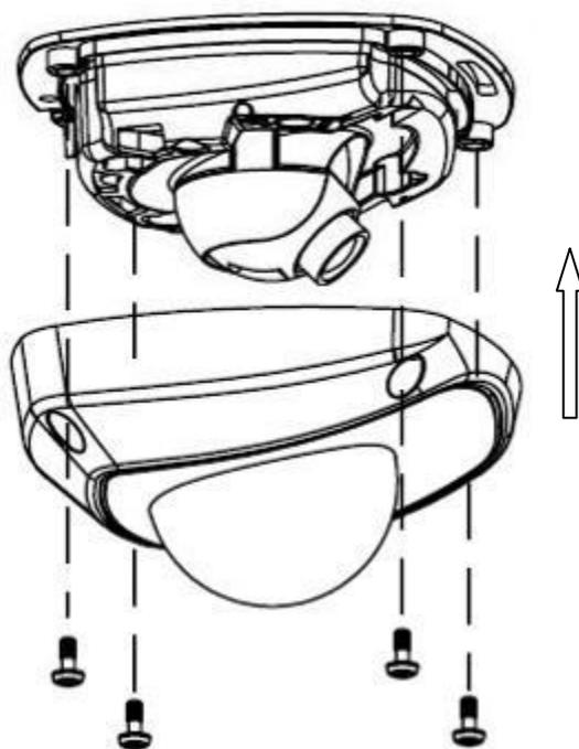
Figure 3.5.7 Install the back box
