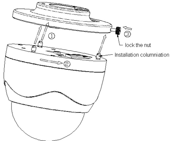
Figure 3.2.2 Dome camera fixing
