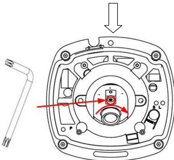
Insert the hexagonal screw driver into the hole marked in the picture , and then adjust horizontally and vertically the camera's pan and tilt by turning the hexagonal screw driver.
