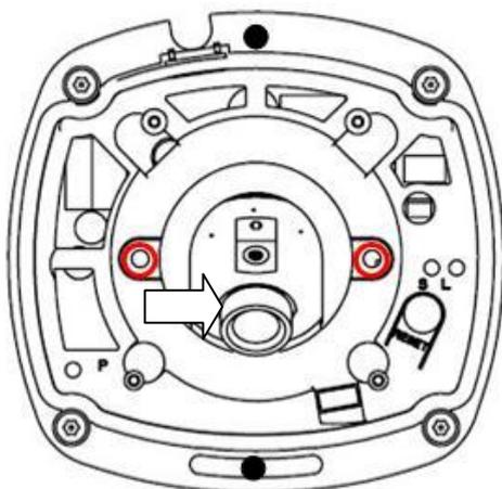
Loosen the lens set screws.
