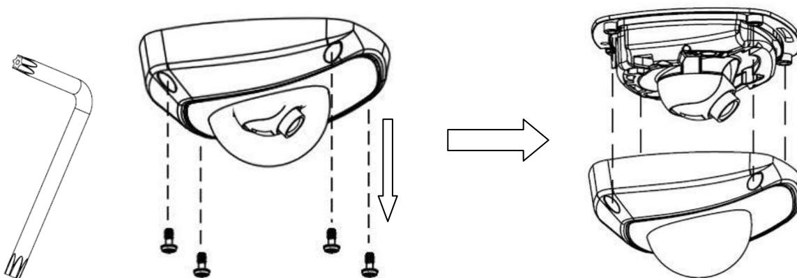
Figure 3.5.2 Remove the back box
