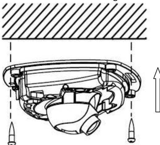
Figure 3.5.3 Fix the bottom board
