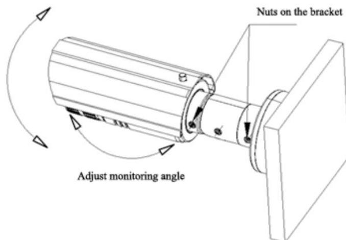
Fig 3.3.3 Adjust monitoring location
