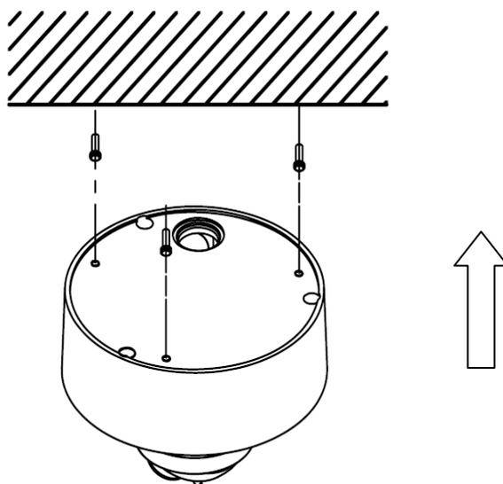
Figure 3.2.5 Install the Camera
