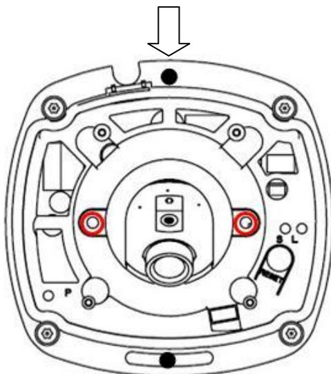
Tighten the lens set screws.
