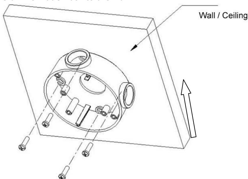
Fig 3.3.1 Fix camera wire hidden box
