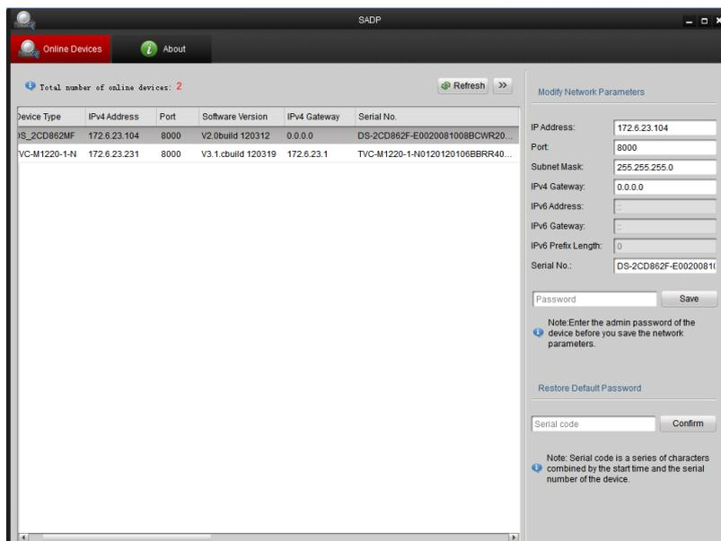
Figure 2.3 Modify Network Parameters
