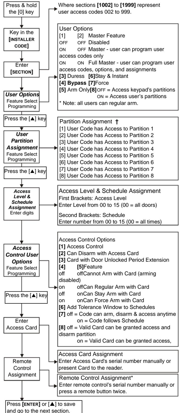
† The default setting depends on the programming user's assigned partitions. For example, when a user (with master feature) that is assigned to partitions 1 and 2 programs a user code, partitions 1 and 2 will be the default setting for the new user.
