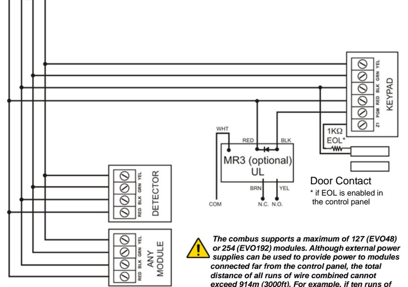
**CAUTION:** The combus supports a maximum of 127 (EVO48) or 254 (EVO192) modules. Although external power supplies can be used to provide power to modules connected far from the control panel, the total distance of all runs of wire combined cannot exceed 914m (3000ft). For example, if ten runs of wire measuring 305m (1000ft) each are connected to the control panel, the total distance would be 3048m (10,000ft), which exceeds the system's capacity.
