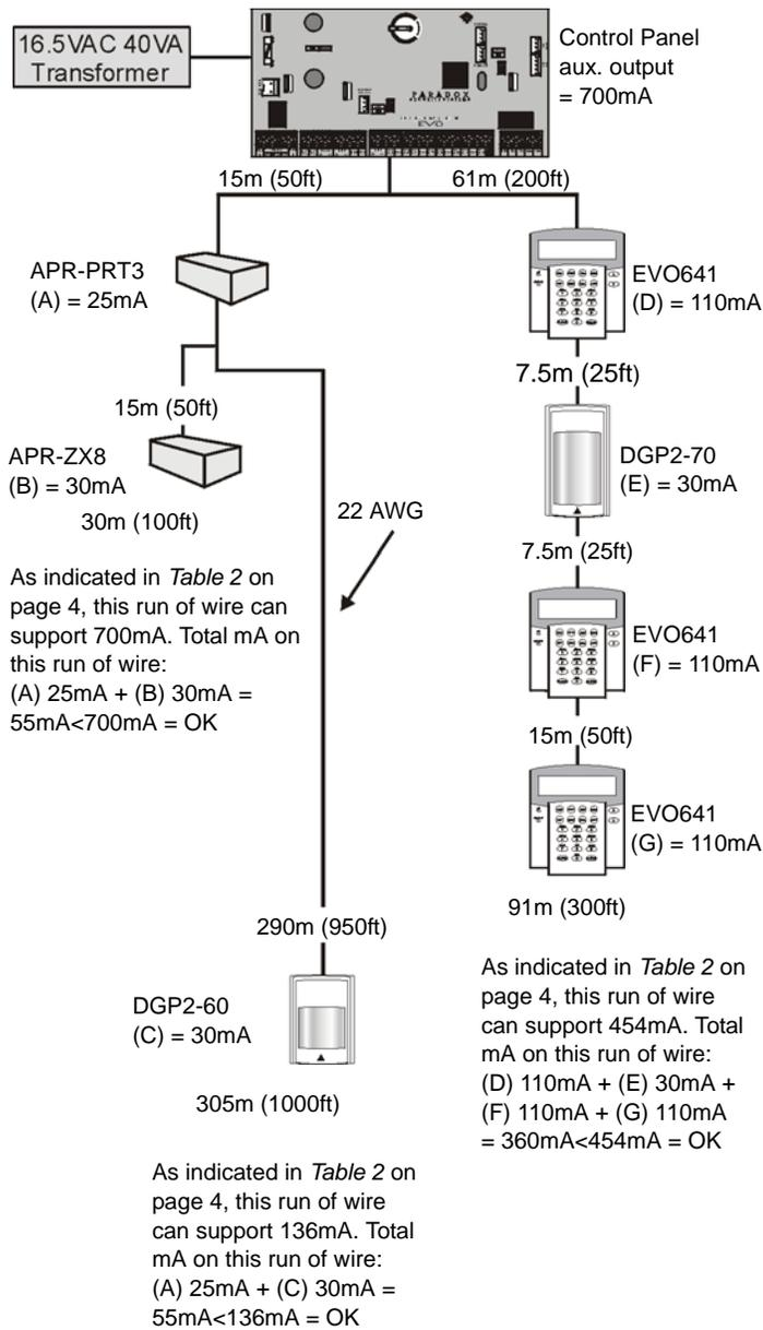
Figure 5: External Power Supply Connections
