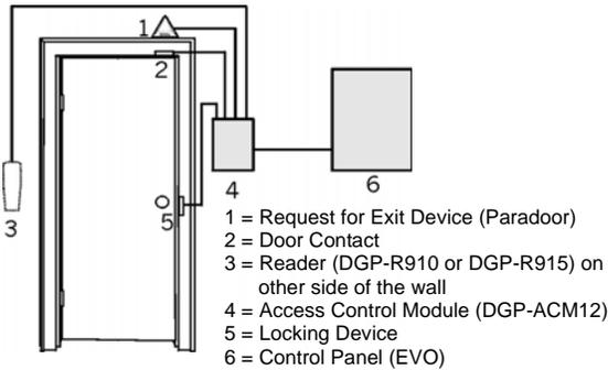
Persons authorized to access the protected area are issued cards assigned to user access codes programmed with an Access Level (see section 15.5) and a Schedule (see section 15.6). The control panel determines whether or not to unlock the door depending on the card's schedule and access.
