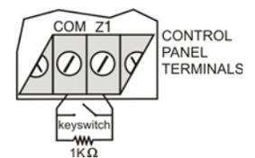
Figure 3: EVO Control Panel Wiring Diagram
