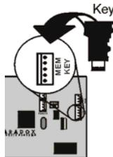
Figure 12: Using the Memory Key
