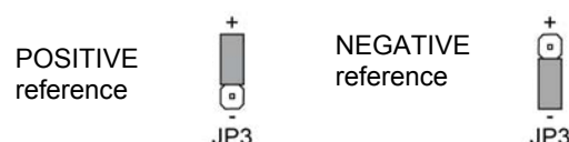
Figure 9 – Electric outputs hardware configuration
