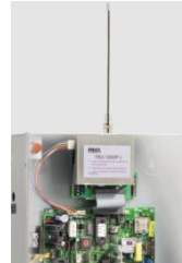
Figure 2. The transmitter mounted in the control panel's box
