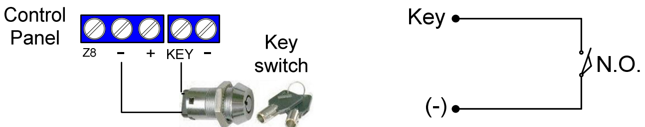
Figure 24. Connecting a key
