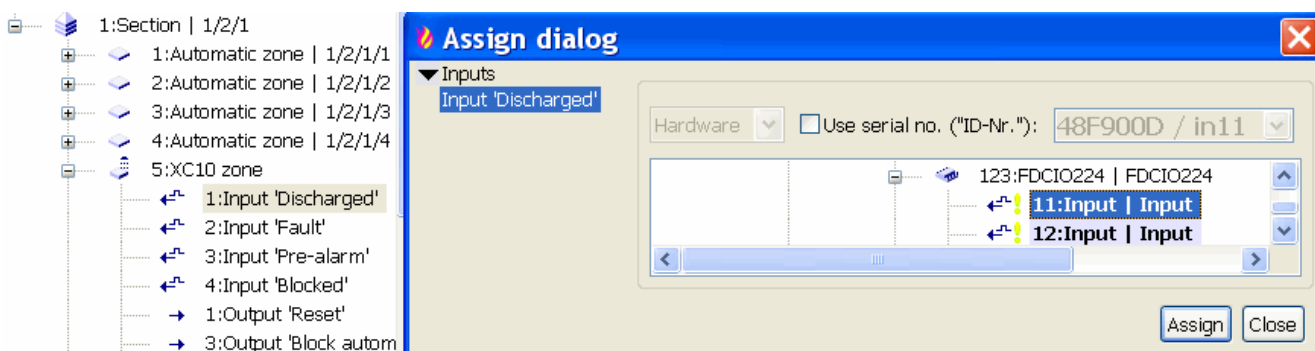
'Assign dialog' window for linking the 'Input discharged' element
