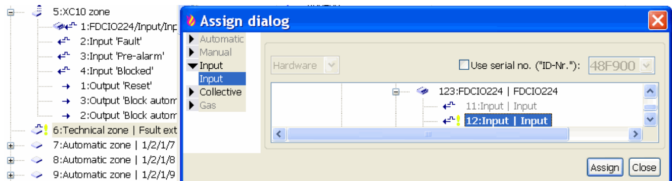
'Assign dialog' window for linking the 'Fault extinguish.' input
