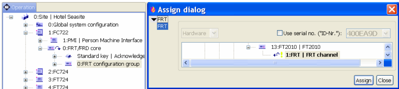
Window 'Assign dialog' for creating and linking the element 'FRT' or 'FRD'
