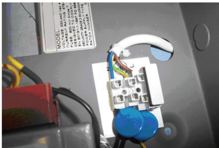
Fig. 21 Cable tie connection to metal indent in base of cabinet
