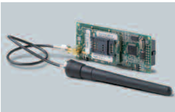
Versatile communications with plug-in GSM and PSTN modules
