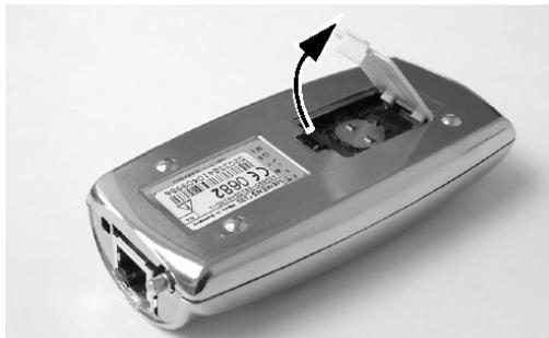
4. Turn the securing plate as far as it will go with the aid of the cover cap:
