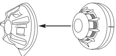
The cover must be removed before the detector is made operational.
