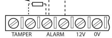
If EOL wiring is not used, the headers should be left in the default (O/C) position. If the required resistance values are not available, leave the headers in the O/C position and wire in external resistors as normal.
