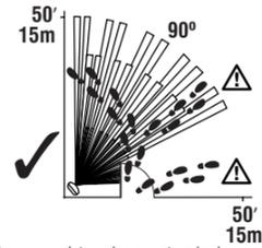
Select the appropriate pulse count and microwave range for the intended installation with JP1 and VR1 and enable the LEDs with JP2. Replace the cover, apply power to the detector and wait 1 minute for the warm-up period to complete.
