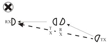
Multi sensors may be used for long-distance guarding. Please install according to the below diagram to avoic interference between beams.
