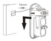
5. Connect the cable to the wire terminal.
