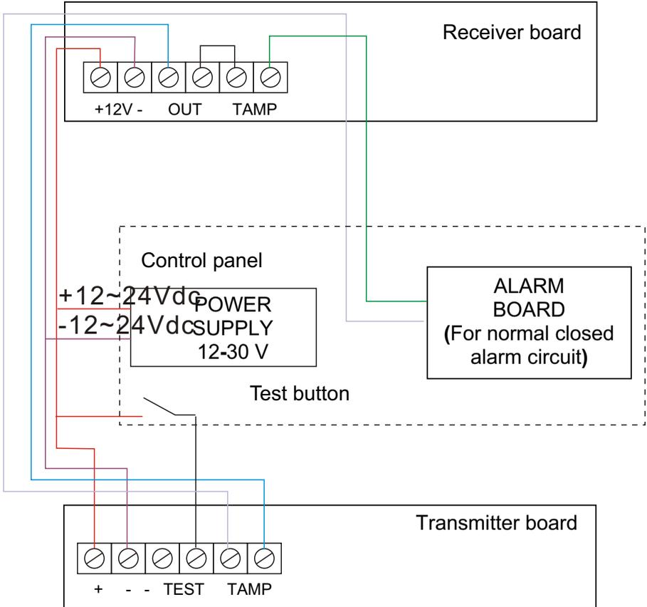
Fig. 6. Control Unit and MCB-200 Wiring Diagram
