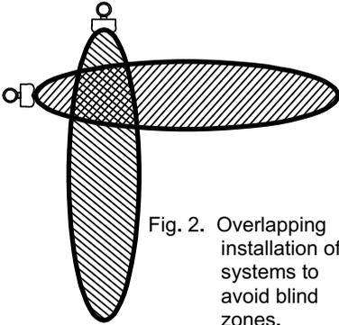
Fig. 2. Overlapping installation of 2 systems to avoid blind zones.
