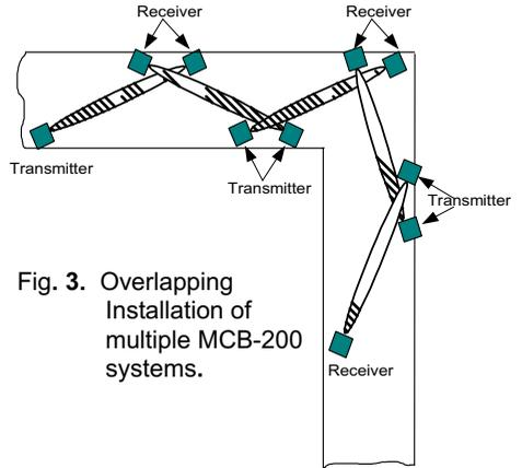
Fig. 3. Overlapping Installation of multiple MCB-200 systems.
