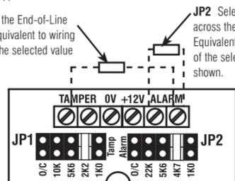
If EOL wiring is not used, the headers should be left in the default (O/C) position. If the required resistance values are not available, leave the headers in the O/C position and wire in external resistors as normal.
