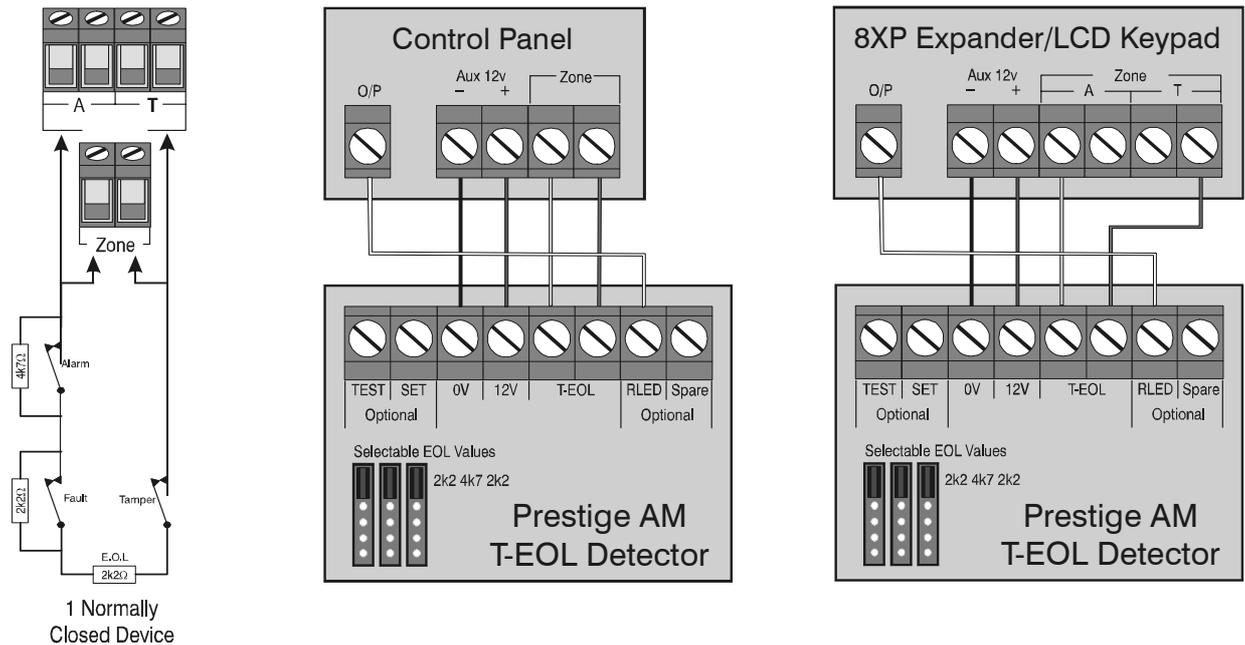
When Configuration Option 13 is programmed as 'Short = Tamper' the system will respond as follows:
