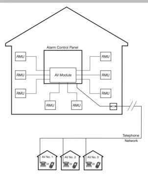
The AV Module will be installed inside the alarm control panel and up to 16 Remote Microphone Units (RMU) will be connected to it. The alarm control panel is connected to the telephone line via a communications module. This allows the system to call up to three recipients (AV No. 1 - 3) following an intruder alarm condition. Once the recipient is connected with alarm system they can listen-in to the protected premises and control the alarm system via a standard touch-tone or mobile telephone.
