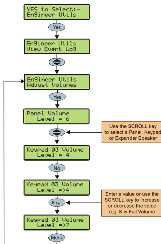
This option is used to adjust the volume level of speakers that are connected to the control panel, keypads and expanders.
