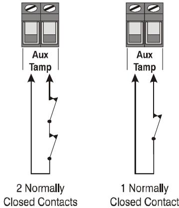
**NOTE** If the 'Auxiliary Tamper' terminals are not being used they must be linked out.
