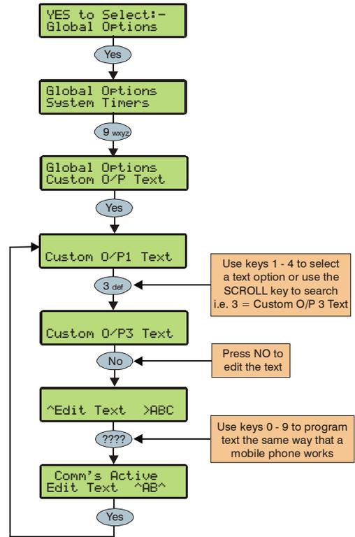
Text may be assigned to Custom Outputs 1 to 4 to allow indication on the keypads display when the output is active (see page 66 for details).
