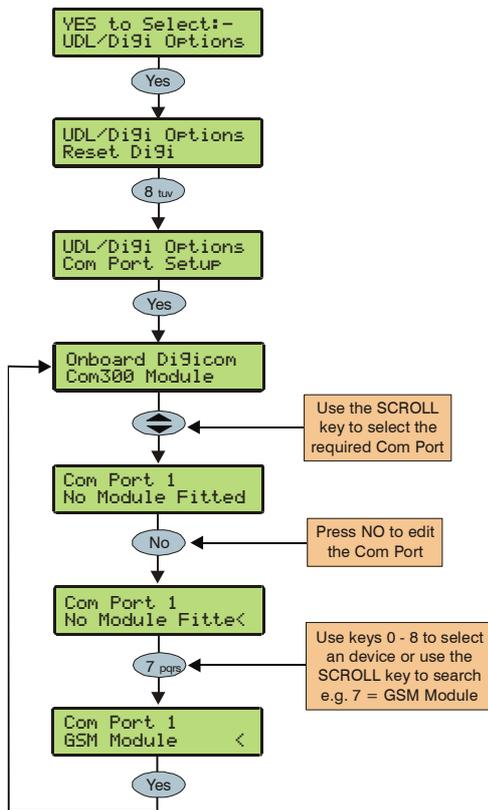
The control panel must be programmed with the type of device that are connected to each of its coms ports.
