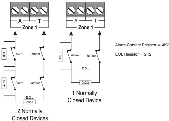
**NOTE** When using this configuration, no more than 3 detectors can be connected to each zone.
