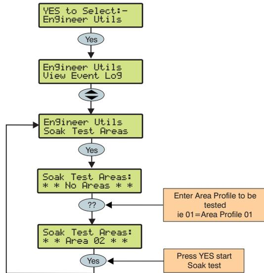
This option allows zones with the 'Soak Test' attribute to be tested by starting the 'Zone Soak Test' timer.
