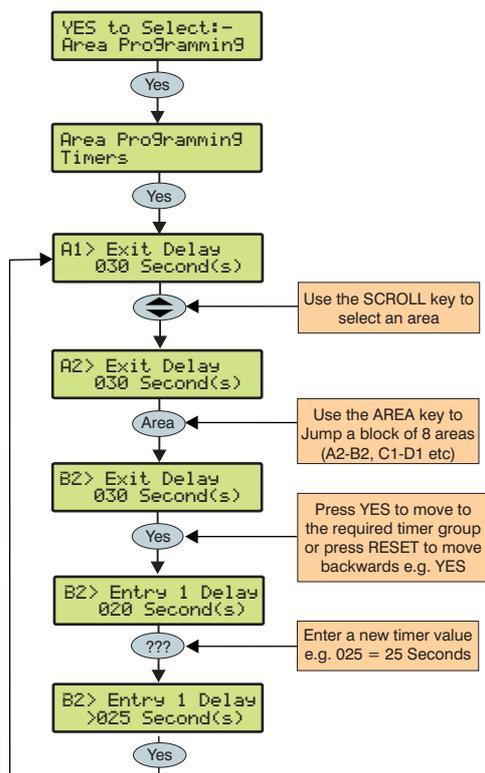
These groups of 'Area' timers control timing and delay functions for areas A1 – H8. Each timer can be programmed for any value between 000 and 999.
