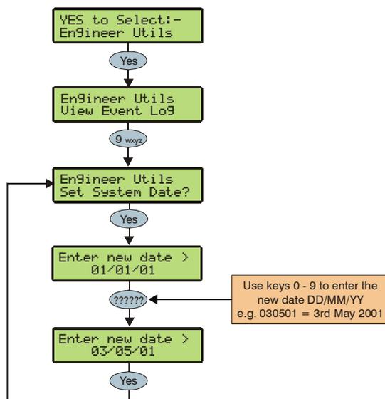
The control panel has a real time clock that is used to date and time stamp events that are recorded within the system log. The option allows you to set the control panel date.
