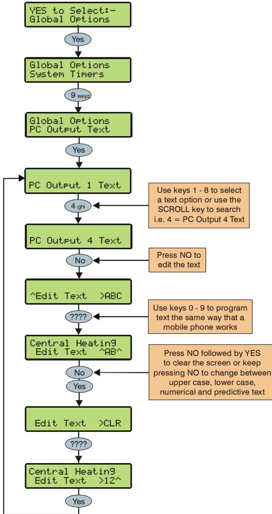
Text may be assigned to PC Control Outputs 1 to 8 to allow the user to select the correct Output by description instead of number. A maximum of 16 characters can be programmed for each of the PC Outputs.
