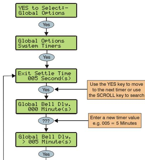
These timers control various timing and delay functions. Each timer can be programmed for any value between 000 and 999.
