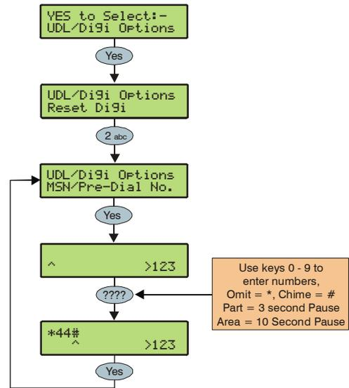
When a *ComISDN* is connected to an extension of an ISDN line with more than 1 number, the direct dial number should be programmed in here, this ensures that the *ComISDN* will only answer a call when the direct dial number is dialled. This number can be up to 24 digits.
