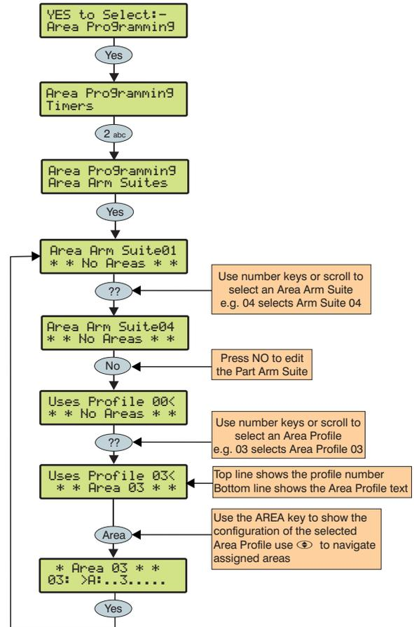
The Premier 640 has 16 Area Arm Suites. Any number of areas can be assigned to each suite via Area Profiles. Assigning an Area Profile to an Area Arm Suite will assign all areas in the Area Profile to the Area Arm Suite. Areas assigned to an Area Arm Suite will be armed when the suite is selected, making it easier for the user to select multiple areas if required.
