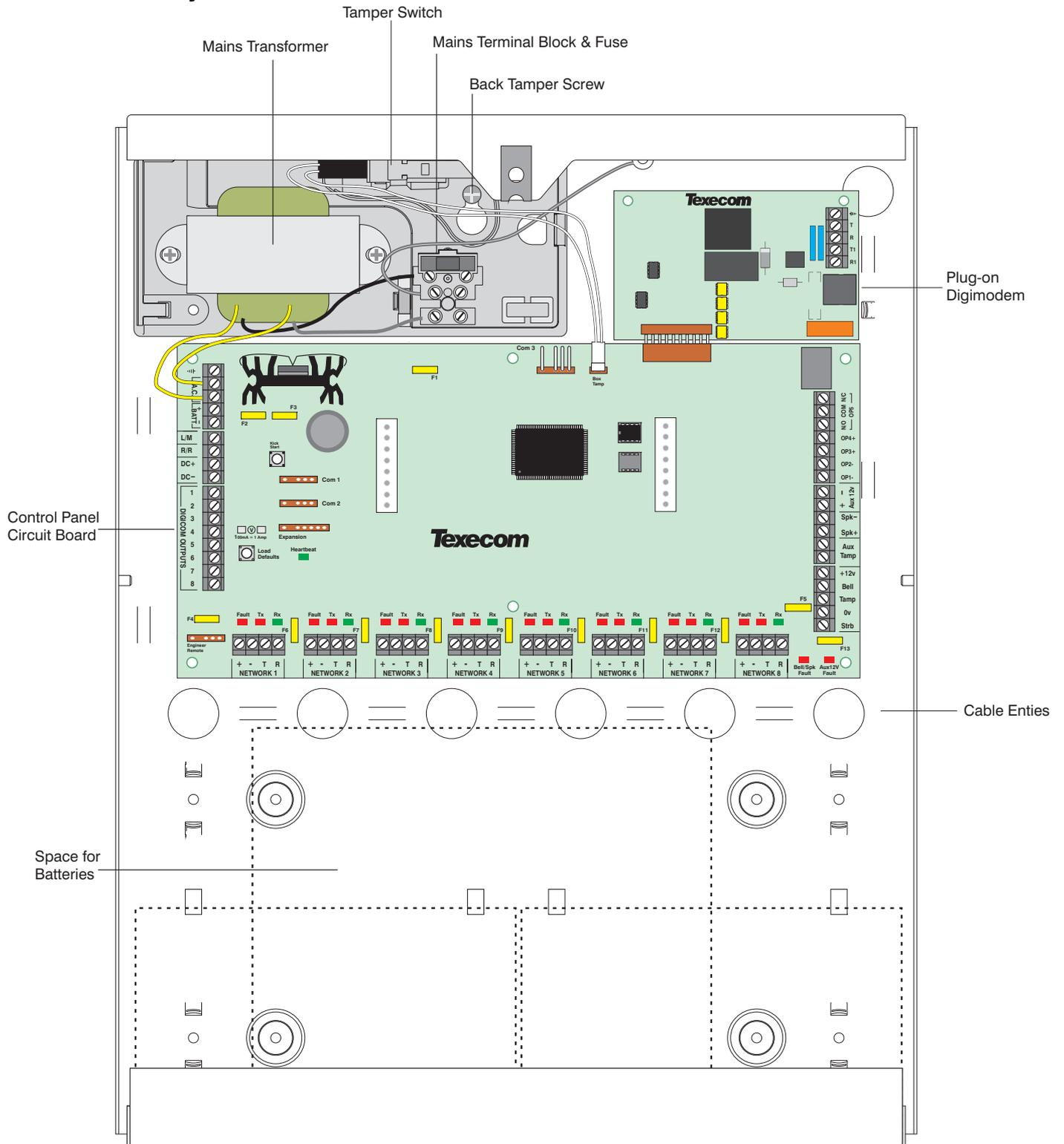
**NOTE** If back tamper is required, the back tamper screw must be fitted as indicated.
