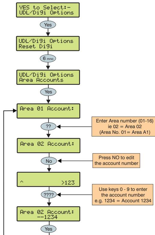
When using Fast Format, Contact ID or SIA, areas A1 to B8 can have their own account number to identify events.
