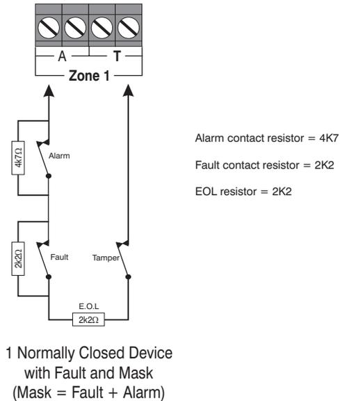
**NOTE** When using this configuration, only 1 detector can be connected to each zone.
