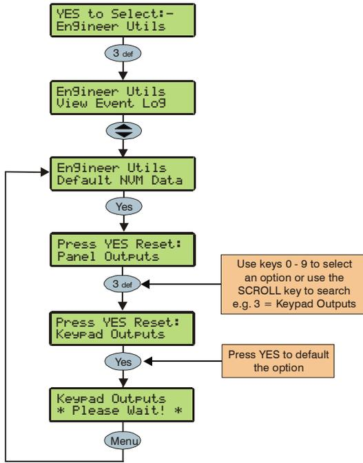
This option allows various parts of the NVM to be defaulted without having to 'Factory Default' the system.
