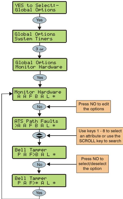
The control panel monitors many inputs for fault conditions i.e. the panel lid tamper, bell tamper, aux fuse etc.
