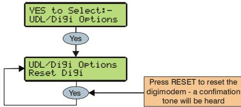
This option should be used whenever a *Premier* plug-on communicator is plugged on or removed from the control panel.
