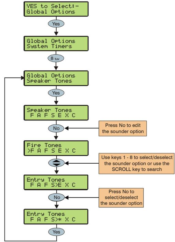
The speaker output on the control panel can be programmed so that certain types of tones are not generated. When deselected, Fire, Alarms, Fault, Service, Entry, Exit and Chime tones will not be heard.
