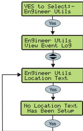
This option allows the 'Panel Location' text that has been programmed in 'System Text' to be displayed (see page 53 for programming details).
