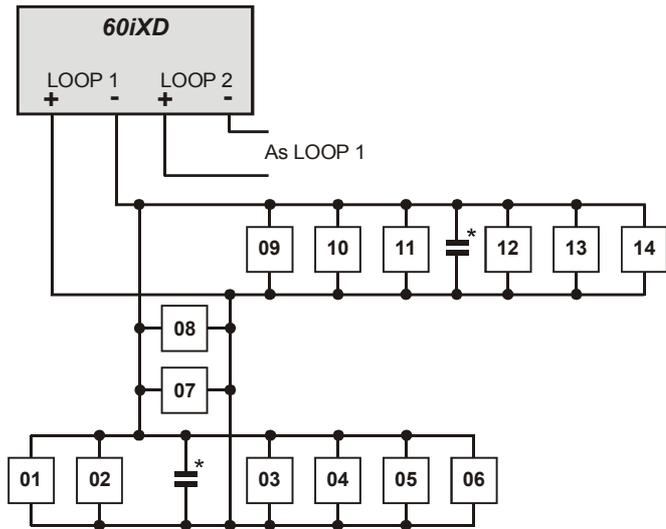
\* The 60iXD expander module is supplied with 4 off 10nF capacitors in the spares pack. It is recommended that you connect a 10nF capacitor approximately at the half way point of each iD spur. It is especially important to do this on iD spurs that are less than 30 metres.
