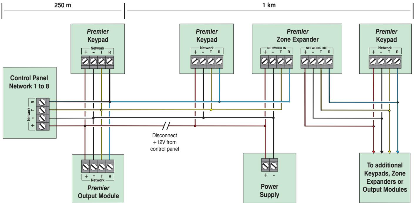
Figure 2: Network Connections (1km with additional power supply).
