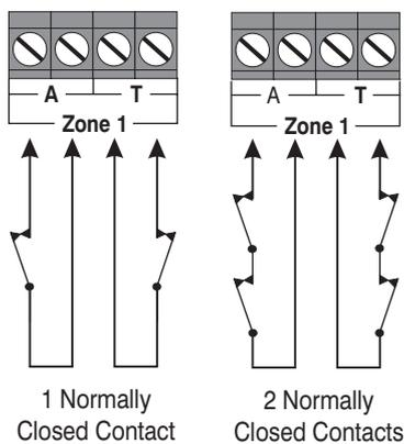
**NOTE** When using this configuration, no more than 10 detectors can be connected to each zone.
