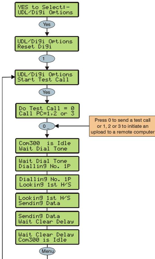
When a *Premier* plug-on communicator has been fitted to the control panel. This option can be used to send a test call to the Alarm Receiving Centre or to initiate a remote Upload/Download call to one of the programmed callback numbers.
