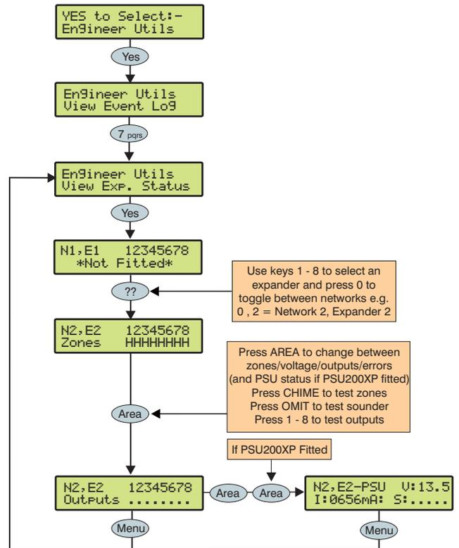
This option allows the status of the expander, the zones, voltage/inputs and outputs and any monitored power supply to be viewed.
