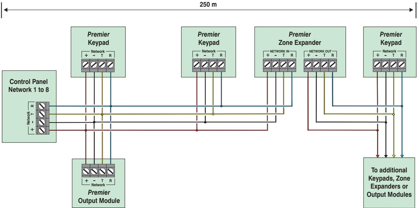
Figure 1: Network Connections (250m without additional power supply).
