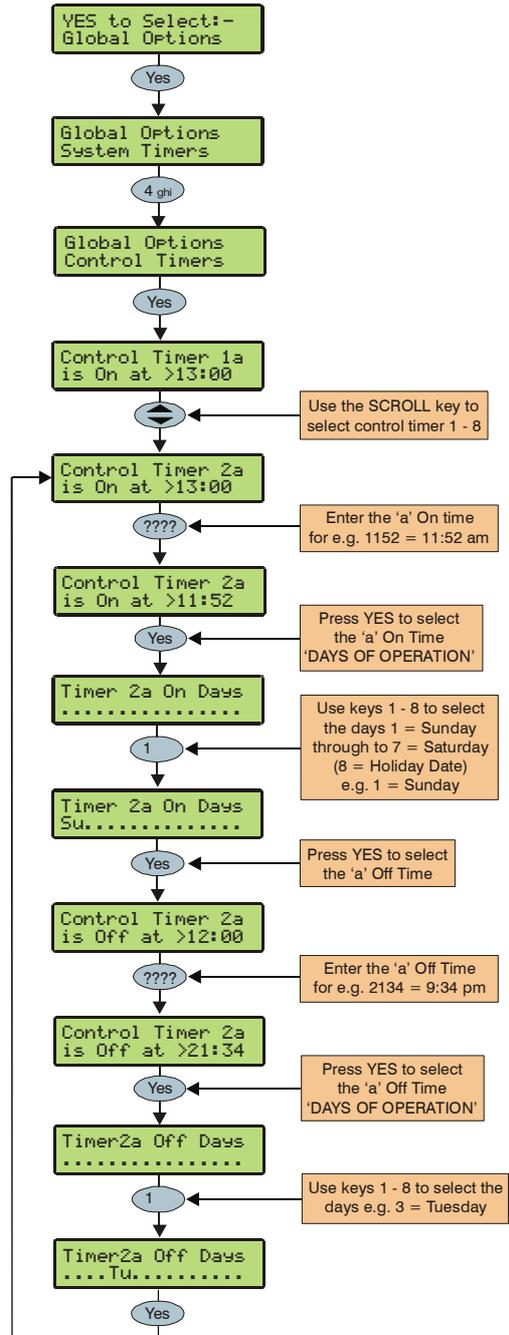
The Premier 640 has 8 control timers. Each timer has two ON and OFF times (a & b), and can be programmed to operate on any day of the week. Once configured, the timers can be used to arm or disarm areas, lockout users and control outputs.
