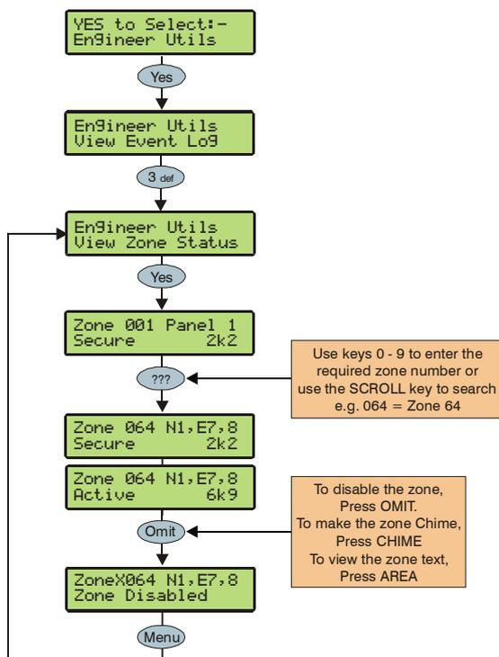
This option can be used to view the status of any zone on the system to see whether it is 'Active', 'Secure', 'Tampered' or 'Shorted'. The selected zone can also be temporarily disabled (zone and tamper) to allow the zone to be worked on or made to chime every time it is activated.
