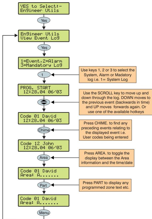
The control panel has three Event Logs, which are time and date stamped. The first log which is a system log, records all events that occur on the system, i.e. Users entering their codes to arm or disarm areas, alarm events, failures to arm etc.
