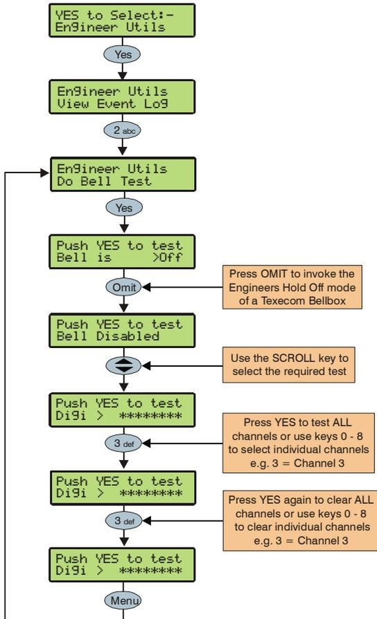
This option allows Allows the Bell, Speaker and various control panel outputs to be tested.
