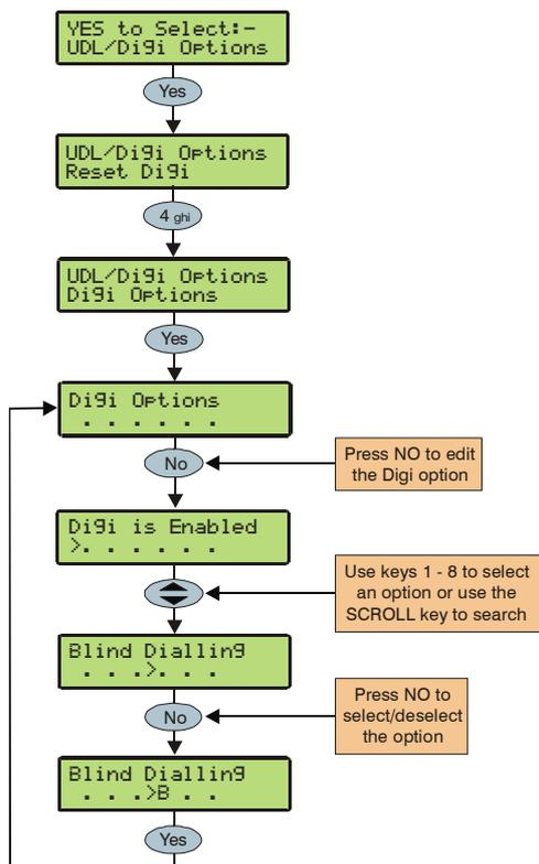
There are 6 options that control how the plug-on communicator works.
