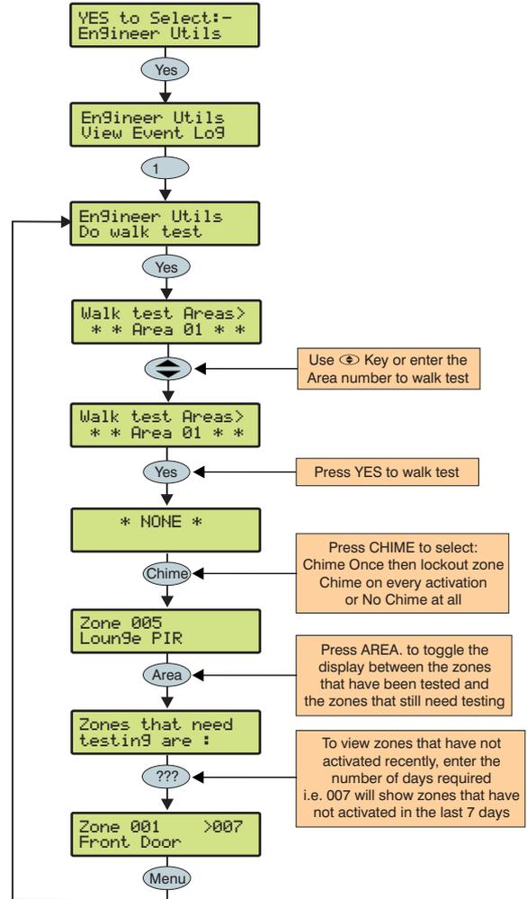
Any of the zones on the system can be walk tested to ensure that they operate correctly. A walk test can only be performed when the system or area is disarmed.
