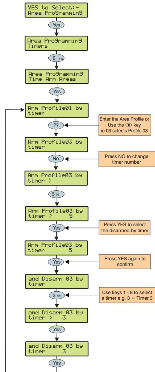
The alarm system as a whole or any number of individual areas can be automatically armed or disarmed using the built in control timers.
