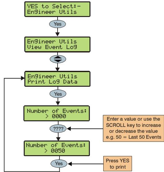
This option allows the 'Event Log' to be printed to a standard RS232 printer (see page 27 for details).
