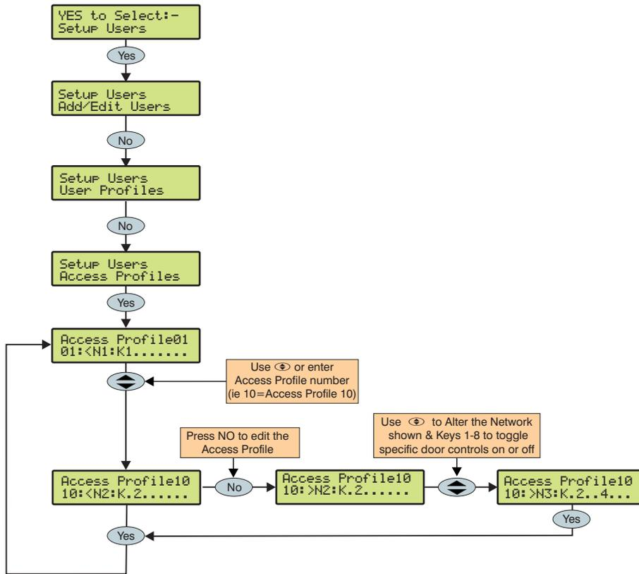
An **Access Profile** determines the doors that a user assigned to the specified **Access Profile** can control. An **Access Profile** can be assigned to any number of users. Once an **Access Profile** has been assigned, any subsequent changes will automatically be applied to all users assigned to the profile.
