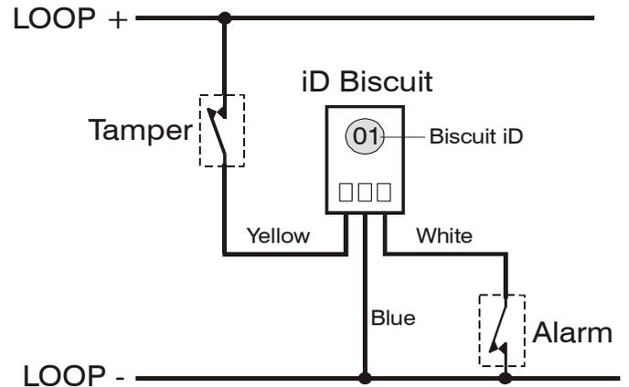
When the tamper switch is opened, the iD biscuit is taken offline and a tamper condition is generated by the control panel. If the alarm switch is opened the biscuit's internal sensor changes state and the control panel will see this as an active condition and will respond as appropriate.
