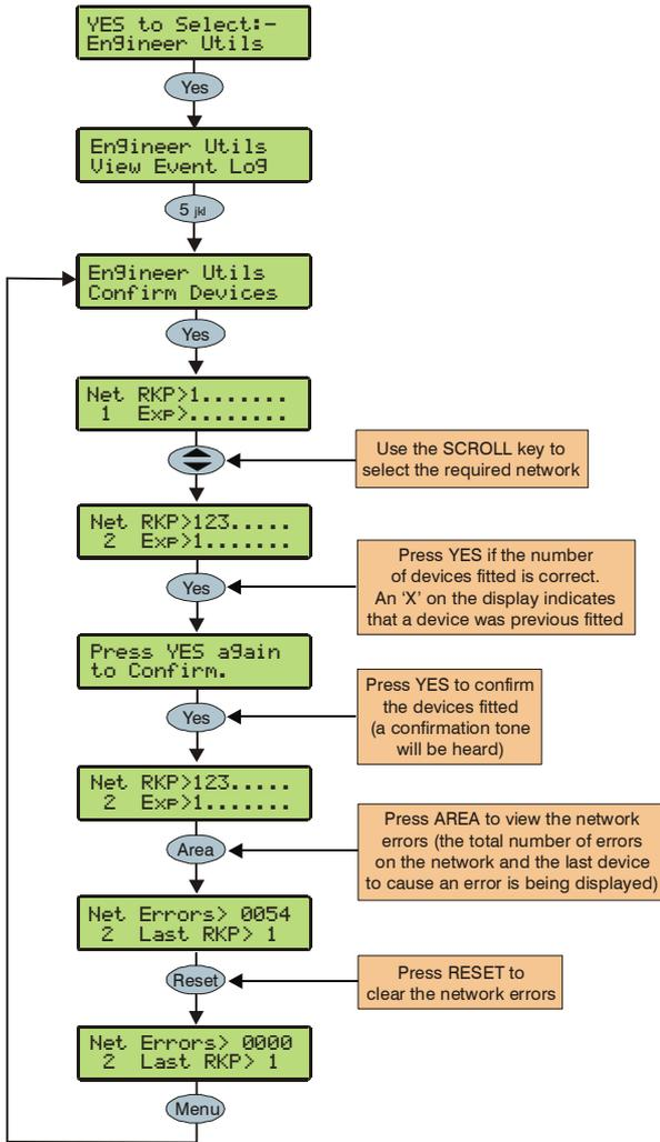
This option allows the networks to be viewed to see what devices are connected and whether there are any problems. Whenever new devices are added to the system, the networks must be checked and confirmed.
