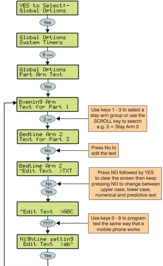
Text may be assigned to Part Arm 1, 2 or 3 to allow the user to select the correct Part Arm by description instead of number. A maximum of 16 characters can be programmed for each of the Part Arms.
