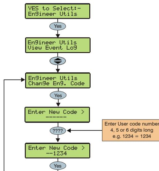
This option allows the Engineer code (User 00) to be changed. This code can be 4, 5 or 6 digits in length. The system will allow a mixture of different length User codes.
