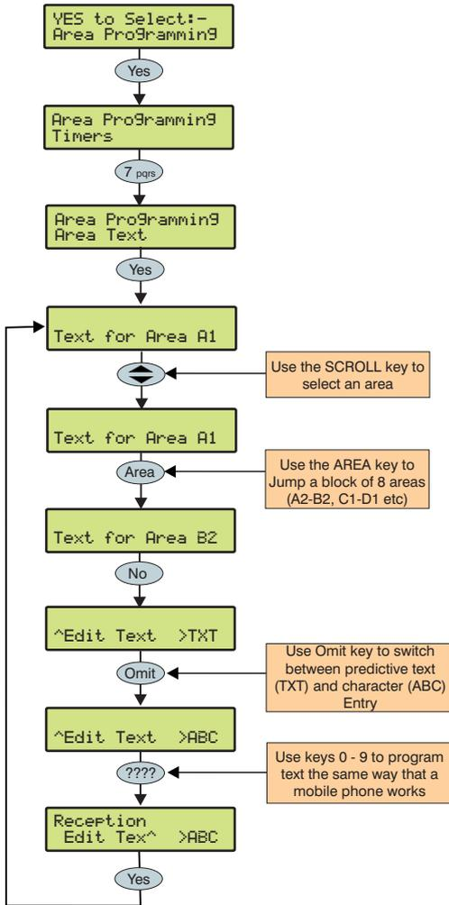
Text may be assigned to each of the areas on the system. This allows the user to select the areas by description instead of a letter. A maximum of 16 characters can be programmed for each of the areas.
