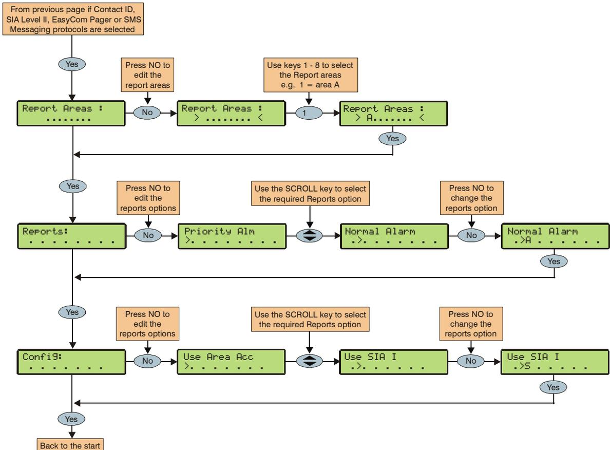
The plug-on communicator can be programmed to dial up to 3 sets of Alarm Receiving Centre (ARC) information. Each 'Set' consists of the following options:
