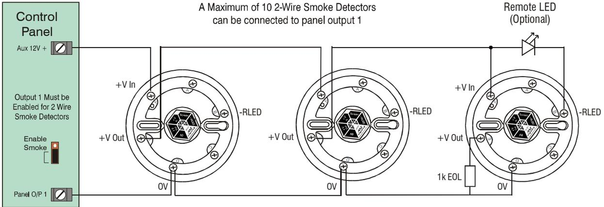
To enable 2-Wire smoke detection on panel output 1, a jumper link must be fitted across the bottom two pins of JP6. The Area Option '2-Wire Smoke' also needs to be enabled (see page 45).
