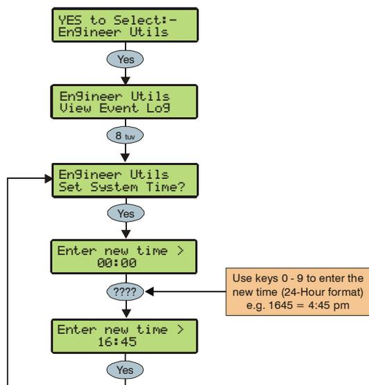
The control panel has a real time clock that is used to date and time stamp events that are recorded within the system log. The option allows you to set the control panel time.
