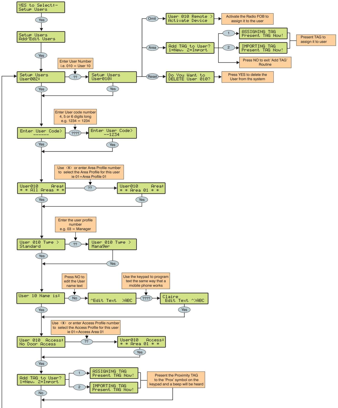
This section covers the alteration of existing users and the addition of new users to the system. The *Premier 640* can be assigned up to 499 users (plus Engineer).
