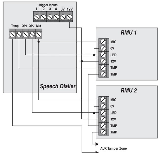
Output 1 (O/P1-) on the *Speech Dialler* is programmed as "Remote Control 1" and Output 2 (O/P2-) is programmed as "Remote Control 2". This will allow the user to switch in and out the *RMU*'s when the *Speech Dialler* is in the Remote Access mode.
