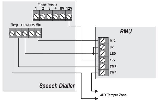
Output 1 (O/P1-) on the *Speech Dialler* is programmed as "Remote Access". This will cause the *RMU* to become active when the *Speech Dialler* is in the listen-in mode.
