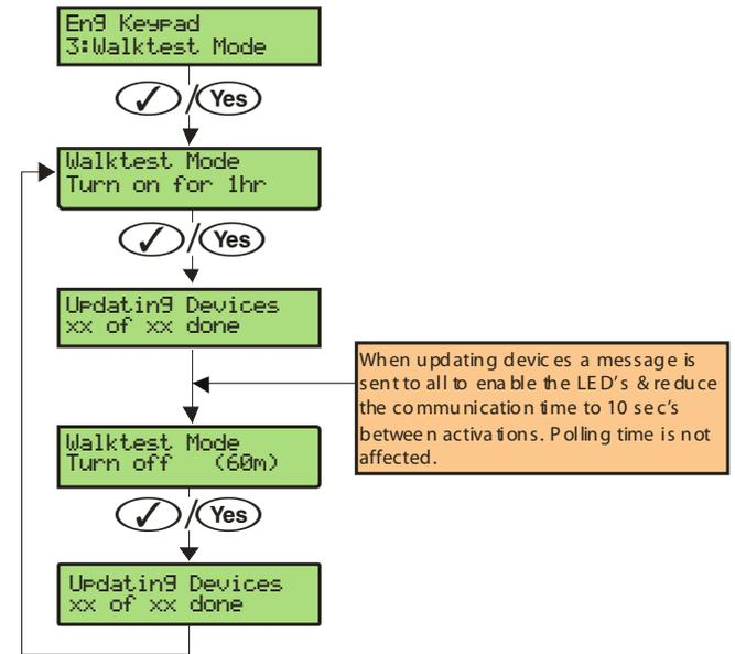
When updating devices a message is sent to all to enable the LED's & reduce the communication time to 10 sec's between activations. Polling time is not affected.
