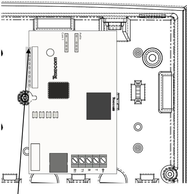
The red lead should be positioned on the uppermost pin of the COM unit.
