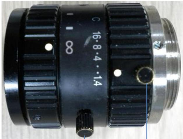
Fixed focal lens has two rotary knobs, the inner is aperture rotary knob, the outer is focus rotary knob. Firstly, adjust the aperture, make sure the brightness of the picture is suitable, then, adjust the focus rotary knob until the picture is clear. At last, lock the focus rotary knob and aperture rotary knob
