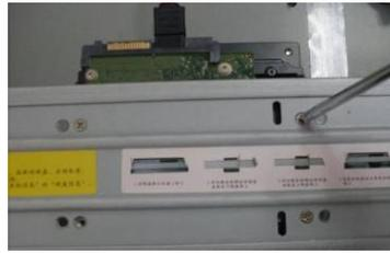
5. Use screws to fix HDD.
