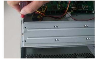
6. Install the upper bracket and then Use screws to fix HDD in the bracket.
