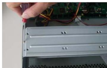
2. Remove the HDD upper bracket
