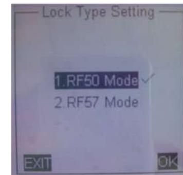
This PDA supports RF57 card (T5557 card), RF50 card (Mifare card). Please select the required type with up and down arrow keys, and then press “OK” button.
