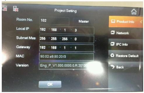
b. Config the network.Here input the IP address of the outdoor station.
