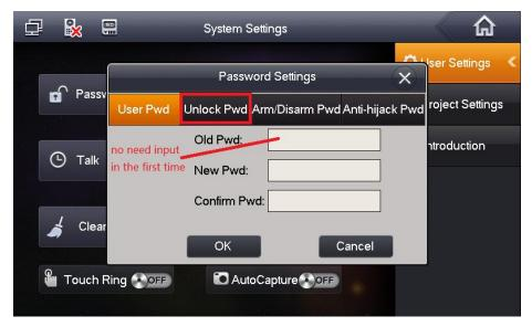
**Step 4** After above settings, user can unlock by self password, on the VTO's panel, user should press # Room No.+ password# to unlock. Please default that the room number should be input as 4 digital. For example
