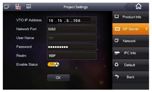
Network>Input VTO's IP address, , point 'OK' to save it
