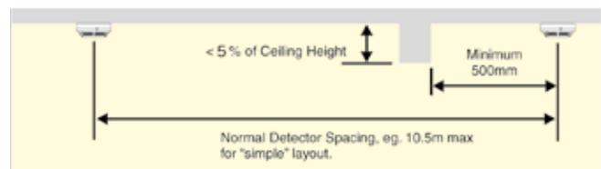
Where a ceiling comprises a series of small cells, for example a honeycomb ceiling, or a series of closely spaced beams, for example floor of ceiling joists, the recommended spacing and siting of detectors changes further, depending on the ceiling height and the depth and spacing of the beams. Reference should be made to relevant standards for details.
