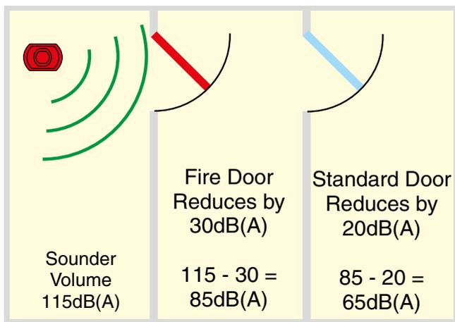
In open space, as the distance from a sounder doubles, the sound level will be reduced by 6dB(A), as shown below.
