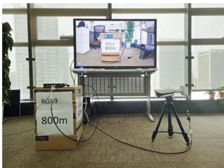
Test of 800m transmission over RG59 cable
