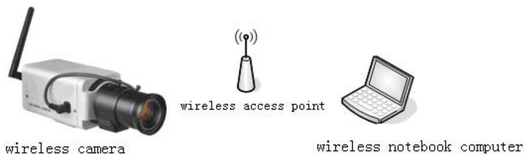
Figure 3.1.2 Connection through wireless access point
