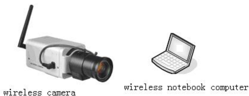
Figure 3.1.1 Point to Point connection
