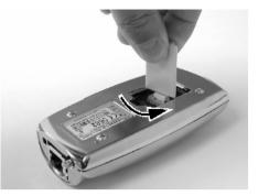
**5.** Flip the holder upwards. Slide the SIM card into the SIM card holder with the contact surface facing down and the flattened side at the top left:
