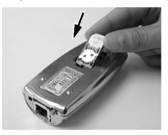
**6.** Press the holder down and secure it with the securing plate. Close the opening with the cover cap.
