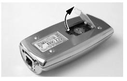
4. Turn the securing plate as far as it will go with the aid of the cover cap:
