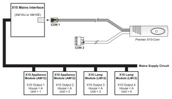
CON1 must be plugged into an X10 mains interface module such as the XM10U or XM10F
