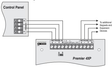
The PCB has a jumper JP2 which allows you to select either STAR (S) or DAISY (D) wiring configuration. The jumper should be set as follows:
