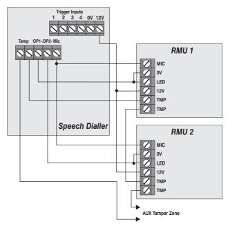
Output 1 (O/P1-) on the *Speech Dialler* is programmed as "Remote Control 1" and Output 2 (O/P2-) is programmed as "Remote Control 2". This will allow the user to switch in and out the *RMUs* when the *Speech Dialler* is in the Remote Access mode.
