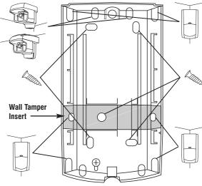
For rear/wall tamper - fix both the detector AND the wall tamper insert to the wall.
