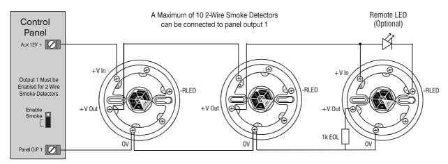
To enable 2-Wire smoke detection on panel output 1, a jumper link must be fitted across the bottom two pins of JP10. The Area Option '2-Wire Smoke' also needs to be enabled (see page 6).
