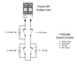
When the Auxiliary Input is programmed as 'PSU Monitor' the system will respond as follows:
