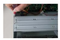
2. Remove the HDD upper bracket
