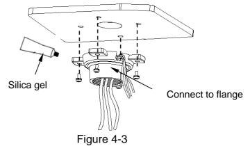
Pull the cable through the steeve and then secure the steeve to the flange. Fix the M4 bolt. Please note, if the speed dome is installed in the outdoor environments, you need to paste enough Teflon tape at the top screw thread of the steeve and then turn the steeve to the flange firmly. Please paste the silica gel on the steeve connection surface to do the waterproof work. See Figure 4-4.
